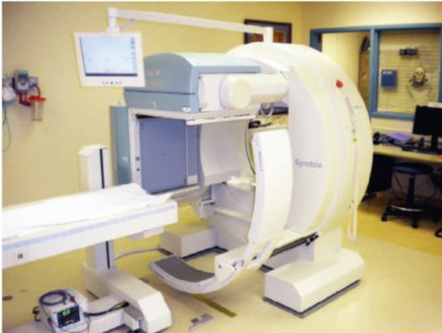
Dual Head Gamma Camera in Cardiac Configuration
