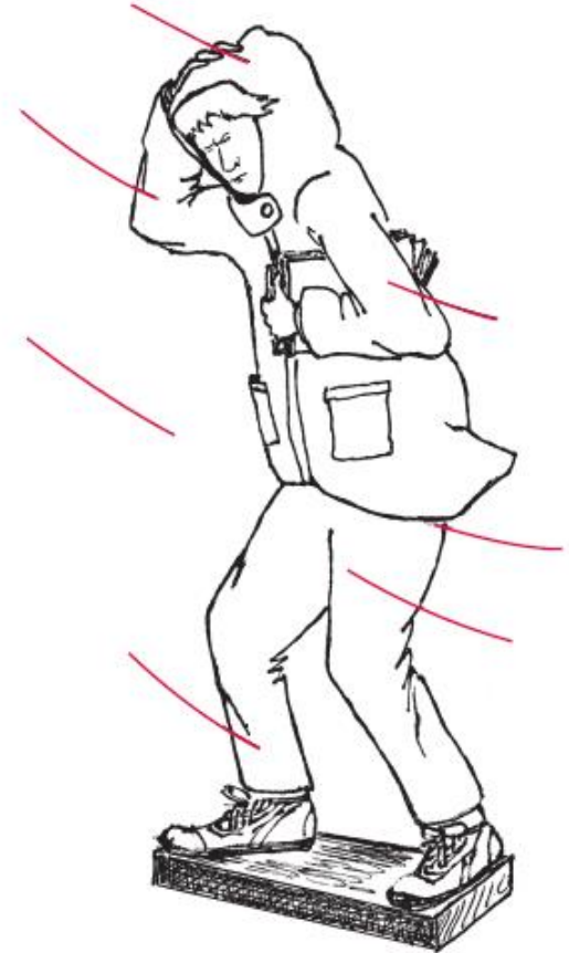
Wider base of support in direction of force increases stability.
